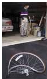
The force of the impact turned the front wheel into a taco shell. Photo courtesy The Chamber Research Used with permission.
