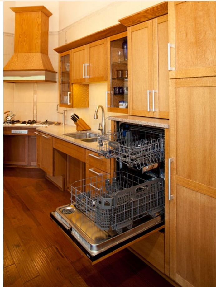
Raised 18 inches off the floor, the dishwasher height is more convenient for both Rosemarie in her wheelchair, and her husband Mark, who is tall.
