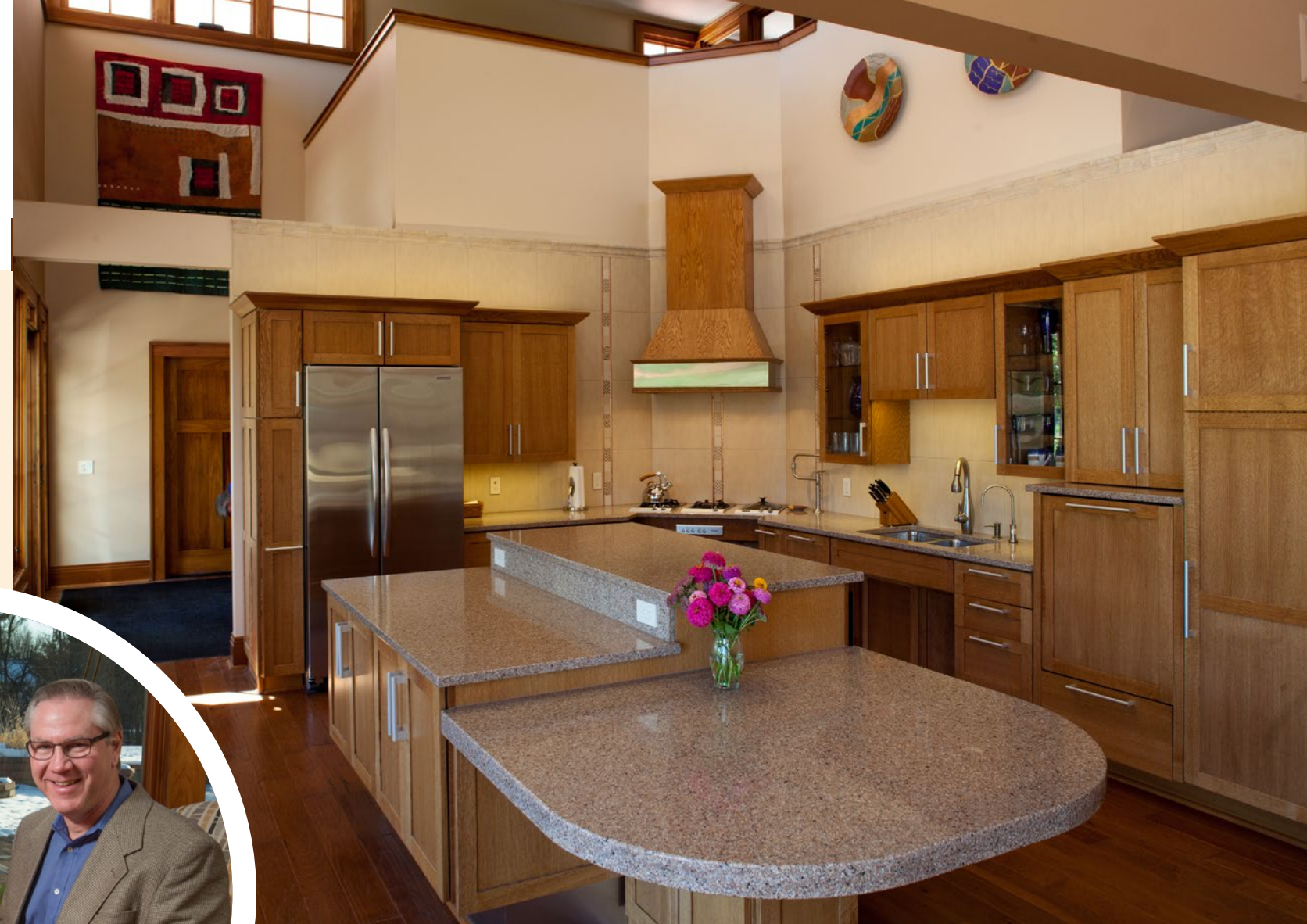
Hardwood flooring, five-foot turning radiuses, and multi-height counters make this spacious home both beautiful and practical.
