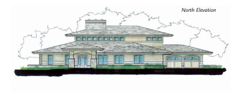
▲ Spread across a level site, the one-story, Prairie Style house has a horizontal rhythm punctuated by high clerestory windows that admit natural light from all sides. The house has no gutters or downspouts to maintain; deep eaves help shade the house and channel rainwater away from the at-grade flat-threshold entries to a fishpond and drainage creek. The front portico extends over the driveway to shield visitors from the elements.
